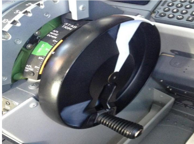
FIGURE 12: THE TRIM WHEEL, WITH THE HANDLE EXTENDED
