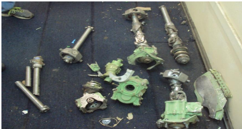
FIGURE47: TRAILING EDGE FLAP TRANSMISSIONS AND BALL SCREWS
