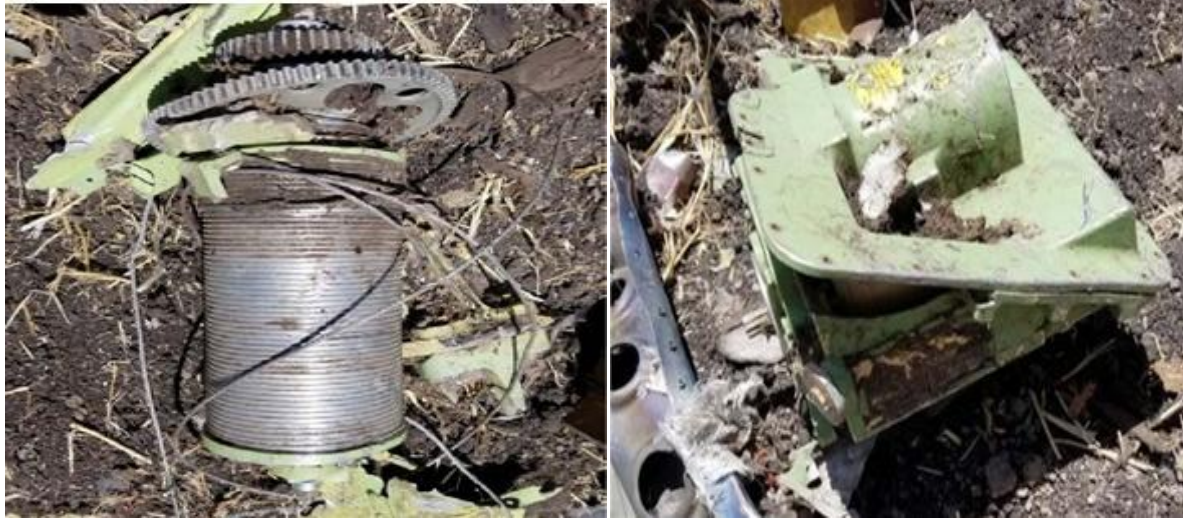
FIGURE 50:AFT CABLE DRUM
