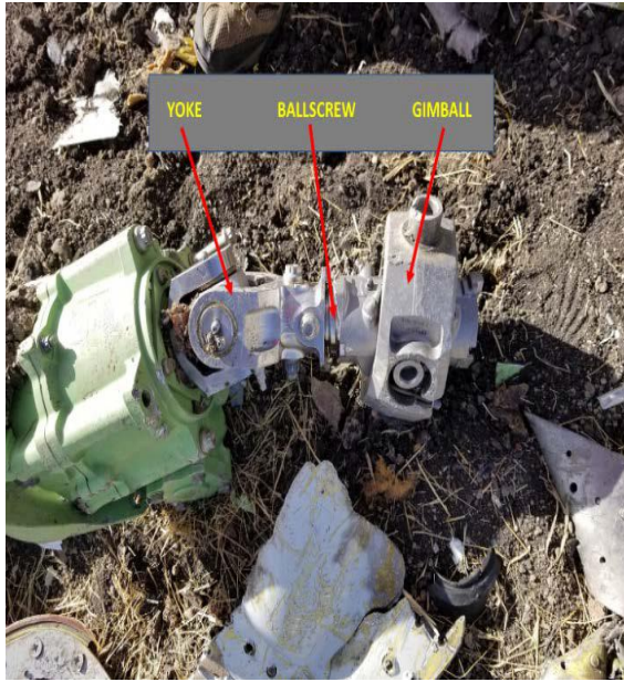
FIGURE45: FLAP TRANSMISSION &amp; BALLSCREW
