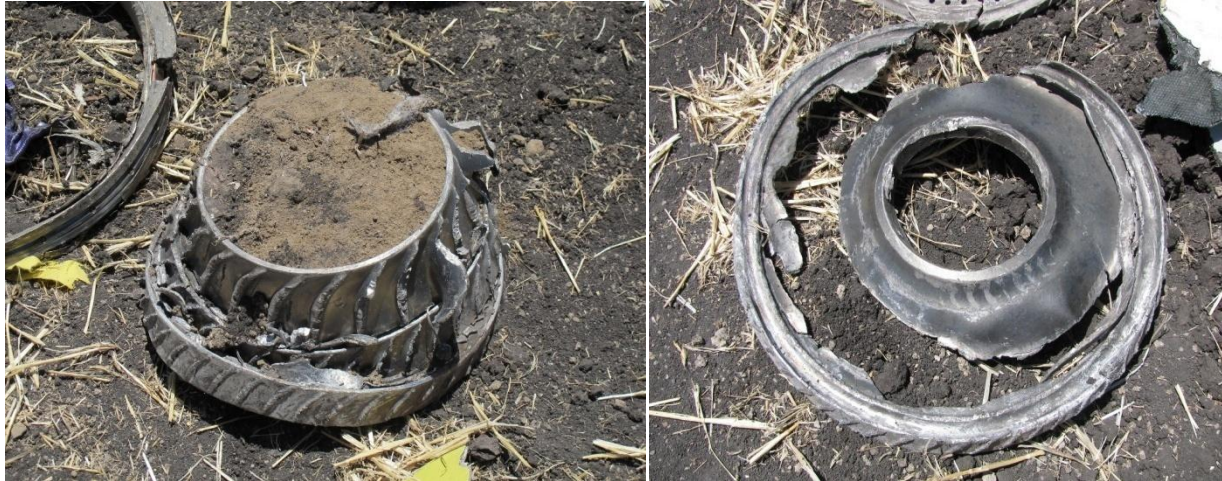
FIGURE 40: - R/H ENGINE - S/N 602695 – HPC STAGES 1 TO 3 FIGURES 41:- R/H ENGINE - S/N 602695 – HPC STAGE 7
