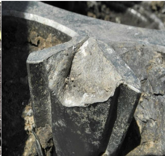
FIGURE 39: R/H ENGINE - S/N 602695 - RETENTION LUGS - FRACTURED
